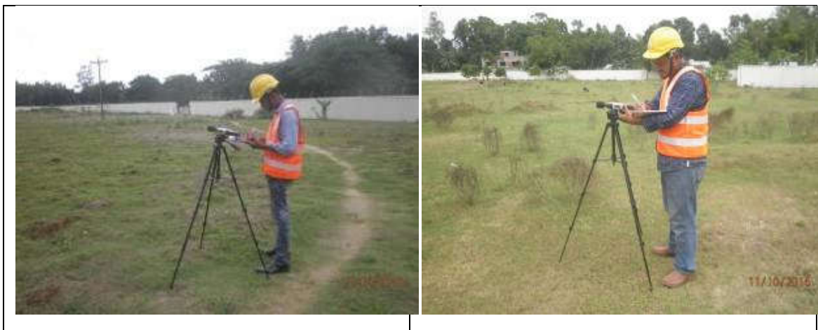
Figure 4.8: Noise Level Monitoring in the Project Area
